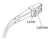
Figure 33. LC-LC Fibre Channel cable lever and latches
